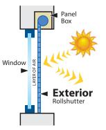
Insulated with a polyurethane foam and mounted on the exterior, rollshutters trap a layer of air between the rollshutter curtain and the window. Both contribute significantly to reducing the cooling and heating energy demand.
