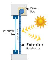
Insulated with a polyurethane foam and mounted on the exterior, rollshutters trap a layer of air between the rollshutter curtain and the window. Both contribute significantly to reducing the cooling and heating energy demand.
